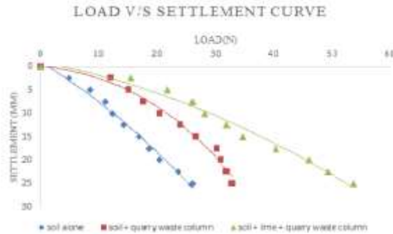
Load Settlement curve for soil bed without column, with quarry waste column and with lime stabilised QW column
